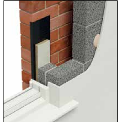
Thermal Cavity Closer MP555 to block return reveal.
