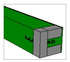
Rather than cutting barriers to size, for example around a window frame, it may be more cost effective to install an 'oversail' end to the barrier at the corner locations. This will not only ensure a tight butt joint is achieved but eradicate the need to cut the horizontal barriers to size.
