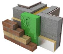
The Masonry **Party Wall Cavity Barrier** is designed to prevent passage of fire through concealed voids within the external fabric of a masonry wall construction, specifically where the junction is formed between the external cavity and the party wall cavity. The polythene-enclosed stone wool fibre barrier is manufactured in bespoke sizes to suit the specified cavity width, and held in place under compression
